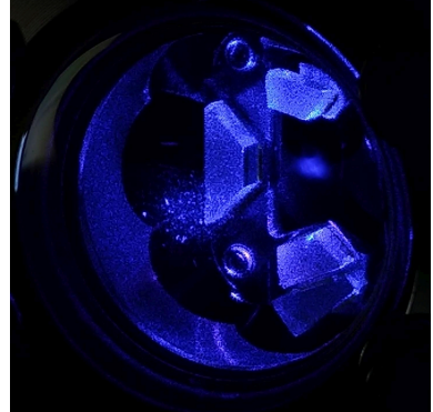
Figure 4.10: Picture of a strontium MOT operated at 461 nm. The atomic cloud, which consists of about 10^6 atoms at 10 mK temperature is visible as a diffuse spot located inside a three-mirror ring cavity (courtesy: Camila Beli and Michelle Moreno).
